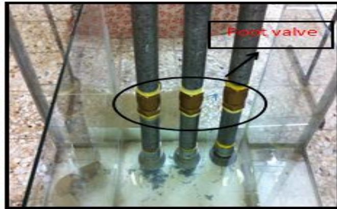
Fig.8. Foot valve used
