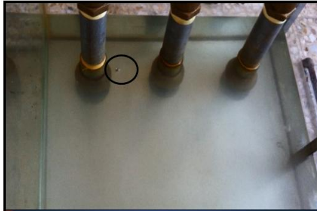
Fig.9. Appearing of vortex type (I-1)
