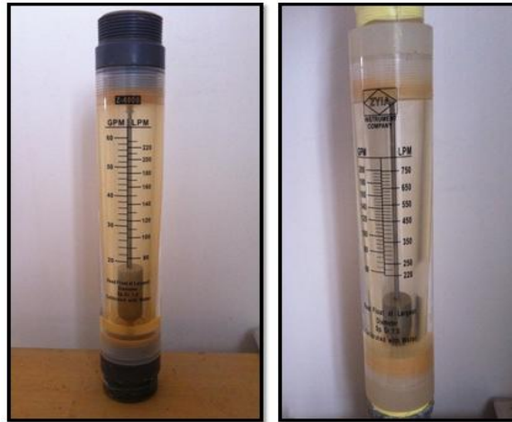
Fig.5. Variable Area Flow meters used
