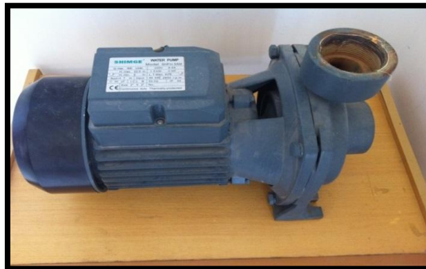
Fig.6. Centrifugal pump used
